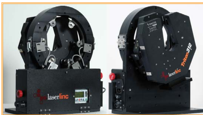
The Profile Vu™ oscillating micrometer fixture (shown here front and back, with two Triton312 micrometers) provides optimal product inspection. The Profile Vu oscillates up to 180 degrees to allow continuous inspection. This fixture is ideal for use in finding width and thickness of non-circular products, such as flat wire, and for locating thick and thin sections of extruded material and other die-formed products.
